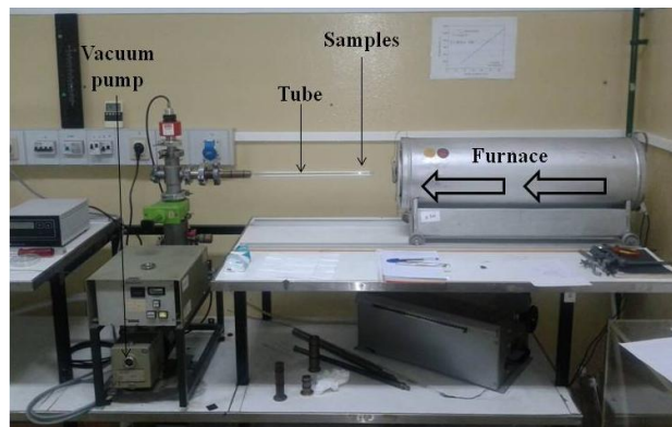
Figure 22. Tubular furnace used for the vacuum annealings.
