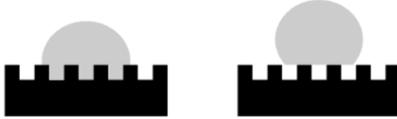
Figure 4. (a) A drop of water in full contact with the surface, according Wenzel model, (b) a drop of water in contact with both air and surface, according with Cassie-Baxter composite model.
