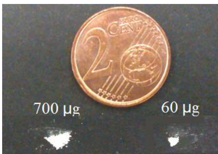
Figure 6.20: Picture of the amounts of particles of SEA 2 and SEA 3, respectively 700 µg and 60 µg, compared with a coin.
