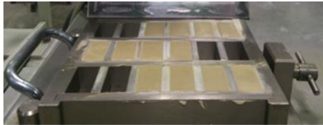
Figure 4-2. Prism mold used in the production of paste samples.
